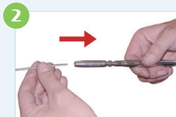
INSERT CABLE INTO FITTING
