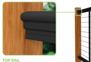
Aluminum top rails can be cut to length in the field and are joined to wood posts using Rail Connecting Brackets (RCBs). Rails easily slide onto RCBs, and are covered with a special snap cap, making installation a snap.
