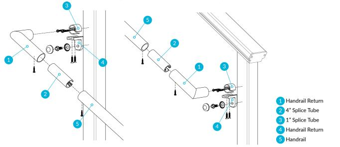
ADA CODE COMPLIANT HANDRAIL (INCORPORATES BOTH TOP AND BOTTOM LOOPED RETURNS)
