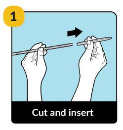
**STEP 1 - Insert cable into needle** Cleanly cut the free cable end and insert it approximately 3/4-inch into the needle hole.
