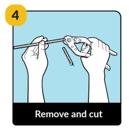
**STEP 4 - Remove the lacing needle** When finished, remove needle and cleanly cut the cable below the kink mark.
