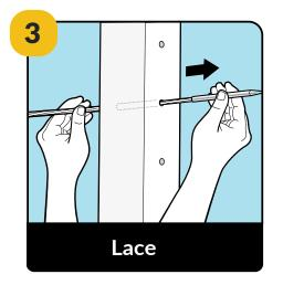
**STEP 3 - Lace the cable through posts** Lace the needle and cable through the post holes.
