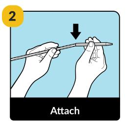
**STEP 2 - Secure the cable in needle** Bend cable to form a slight kink then push it all the way into the hole. The kink will help hold the needle on the cable.
