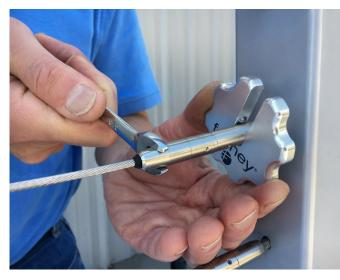
Manufactured from lightweight and durable 6061 aluminum alloy for long-lasting performance, the Quick-Connect® Wrench Wheel allows for continuous full rotation without requiring repositioning of wrenches – making it a faster and easier alternative to the two-wrench tensioning method. The tool utilizes a specially designed spring ball retainer that securely grips onto the wrench flats of the Quick-Connect® Tensioner fittings for ease of maneuvering.
