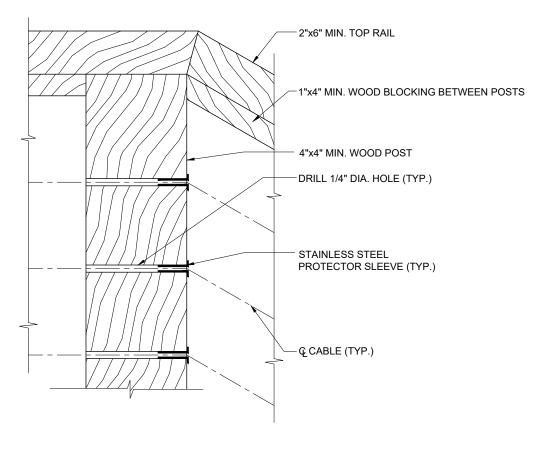
NOTE: INSERT PROTECTOR SLEEVES IN ALL HOLES WHERE CABLE ENTERS AT AN ANGLE TO PREVENT THE CABLE FROM CUTTING INTO THE WOOD. (I.E. STAIR TRANSITION POSTS OR OUTSIDE FACES OF DOUBLE CORNER POSTS)
