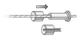
Insert the shaft of the tool into the end of the Quick-Connect® fitting and push firmly to release the jaws. While maintaining pressure on the tool, remove or reposition the fitting as needed. The jaws will automatically re-grip the cable when the tool is removed. Note, if the fitting has a silicone Protection Seal, remove seal prior to inserting the tool.
