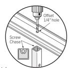
**11) Attach Pickets To Top Rail Insert:** Identify which end is the top end of each picket by comparing the spacing of the first cable hole in each picket to that of the first (top) pre-drilled cable hole on the posts. Use the F screws to attach the top end of the picket(s) to the top rail insert. (**If not using a bottom rails then skip to step 14**).
