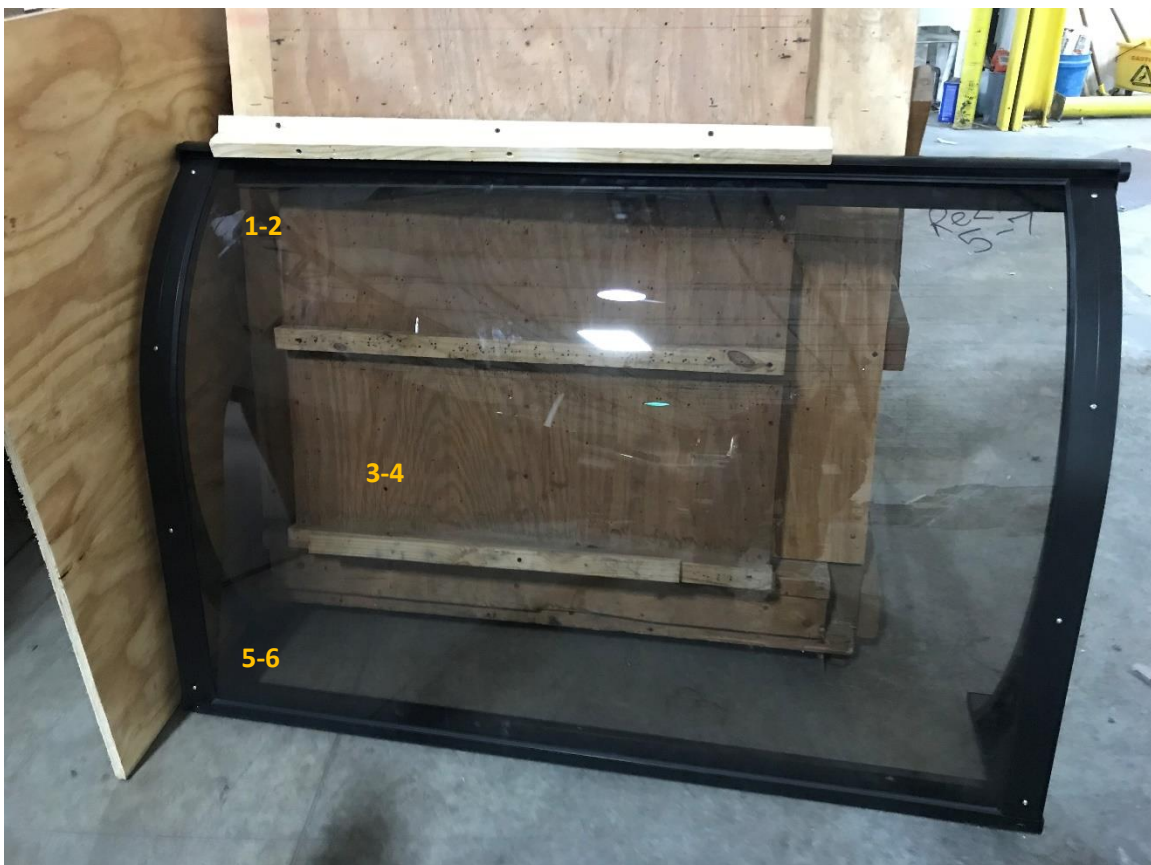
Photo No. 1 Specimen Anchored to Test Deck (Location of Impacts Shown by Numbers)
