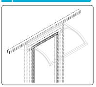
Determine location of awning on wall, and ensure blocking or structure exists at the attachment points. Pre-drill at mounting hole locations, based on specific fastener requirements.
