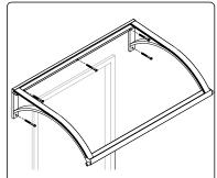
Attach awning using necessary hardware for mounting substrate. Use weatherproof sealant between awning and mounting surface, and along top and side joints.
