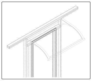
Determine location of awning on wall, and ensure blocking or structure exists at the attachment points. Pre-drill at mounting hole locations, based on specific fastener requirements.
