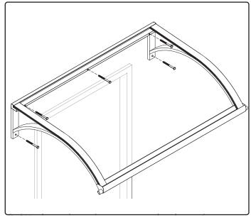
Attach awning using necessary hardware for mounting substrate. Use weatherproof sealant between awning and mounting surface, and along top and side joints.
